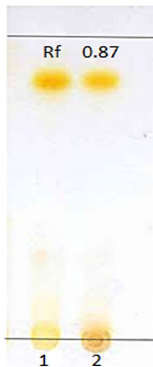
Fig. 3 Thin-Layer Chromatography (TLC) of C. parietis AUCs yellow pigment and standard \beta -carotene using acetone and n-hexane in a 6:4 (v/v) ratio shows bands with an R_f value of 0.87. 1 is the pigment extract and 2 is the standard \beta -carotene
